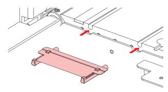
**5** Secure the media holder stopper with the screw.
