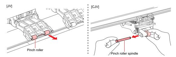
**A** Mount new pinch rollers, and secure them using the O-ring.
