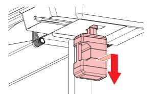
6 Attach the cap to the removed waste ink tank, and use tape to prevent leakage of waste ink.
