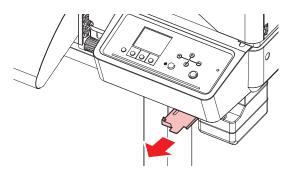
5 Hold the handle on the waste ink tank and slide out.
